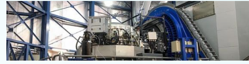
The Cryogenic high-resolution Infrared Echelle Spectrograph (CRIRES+) mounted on the VLT UT3.
